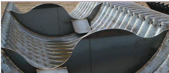
Duguay-Hannaford baffles prior to polymer coating of steel. (Photo courtesy of CSPI)
